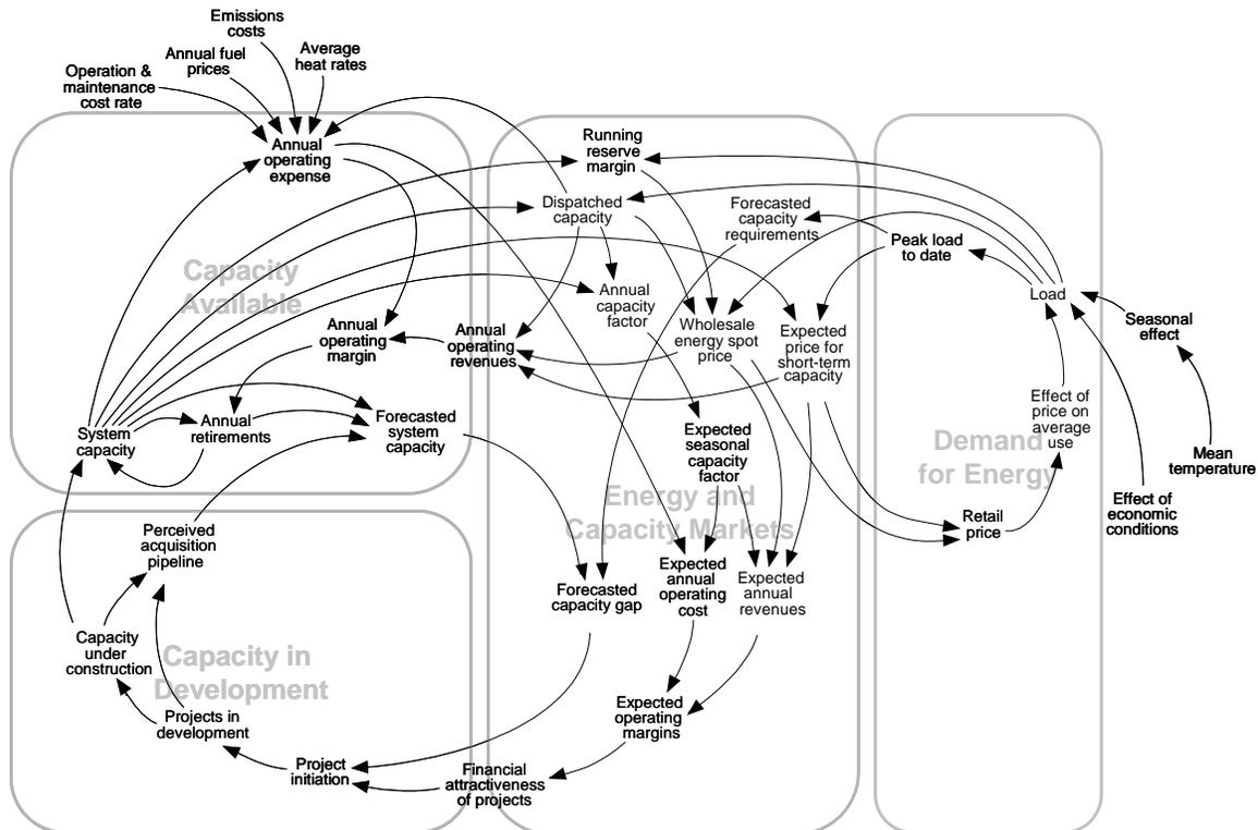
**Figure A.3. More detailed view of feedback loops, in particular the multiple related power and capacity markets, and the expectations formations that drive investment in power plant construction projects.**
